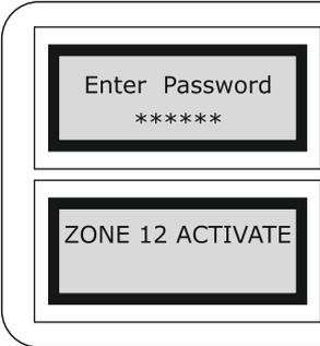
To activate the dialer press **F3** key and type six digit password "\*\*\*\*\*" and press **ENT** key.
