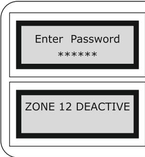
To de-activate press the password directly "\*\*\*\*\*" **ENT** key.
